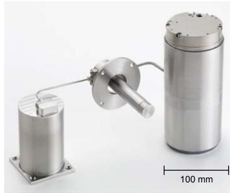
Fig. 12 Components of the SWIR camera system. The integrated detector cooler assembly (left) houses the MCT photodiode array, the ROIC and the pulse tube cooler in a compact dewar. For the picture the top part of the dewar including the cold shield and the optical interface were omitted. The cooling system (right) is composed of a pulse tube cooler driven by a symmetric compressor for low residual vibration output. Pictures courtesy of AIM [6].
