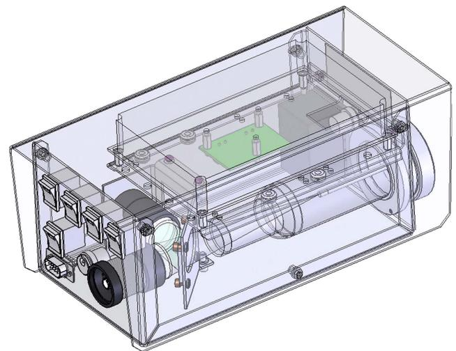
**Figure 6.** Transparent view of the eShel calibration unit (Shelyak Instruments). (A color version of this figure is available in the online journal.)
