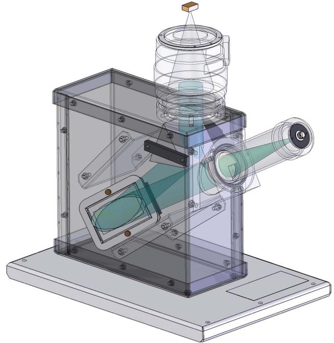
**Figure 5.** Transparent view of the eShel spectrograph (Shelyak Instruments). (A color version of this figure is available in the online journal.)
