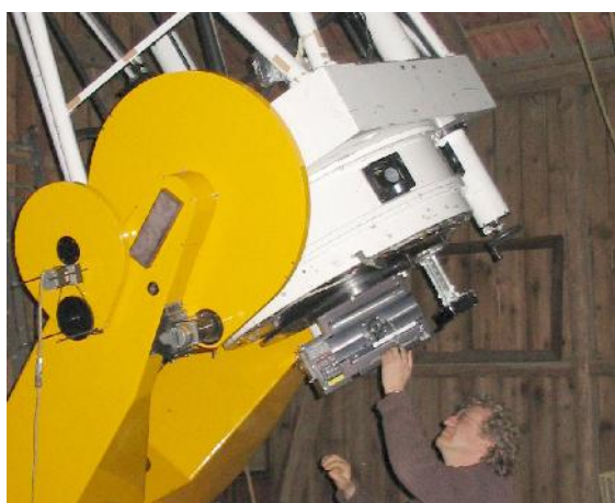
Figure 13: The STScI main instrument. Two of the four cooling fans for the primary mirror are visible on the mirror cell (STScI).
