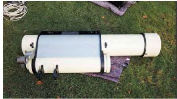
A 20 cm f/10 folding refractor according to Günter D. Roth
