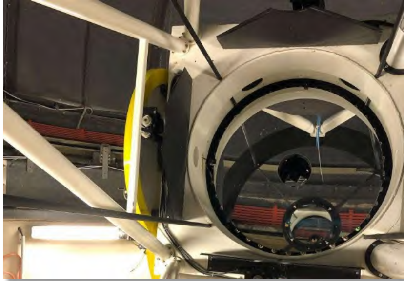
View of the primary mirror in the telescope. The mirrored secondary mirror can be seen below the mirror opening.
