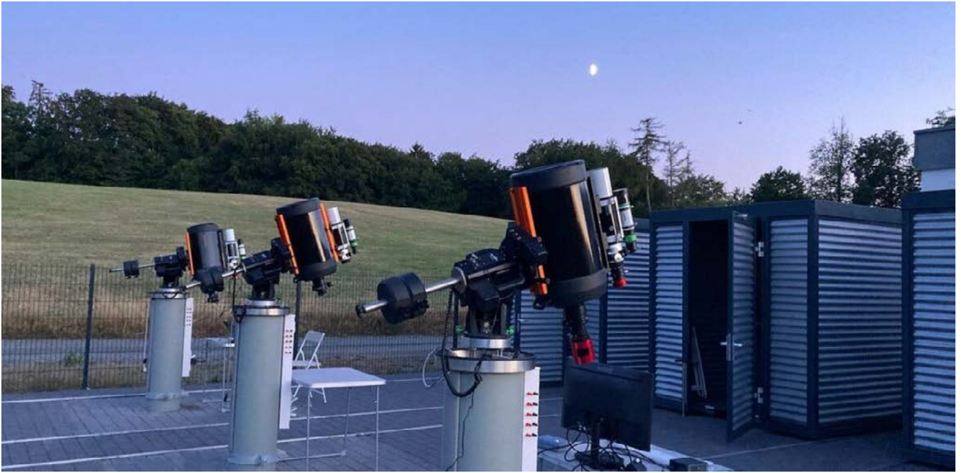
2 The school laboratory with three identical 28 cm telescopes. The sliding steel 'cubes' can be used as heated control rooms.
